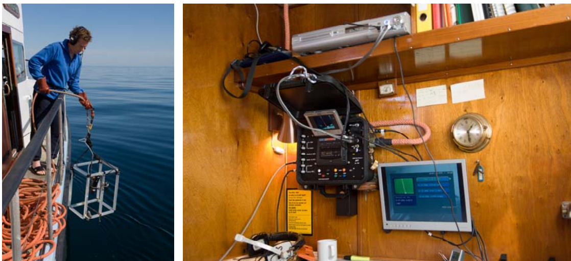
Figure 6. Underwater video system with monitor and hard disk/DVD recorder.
