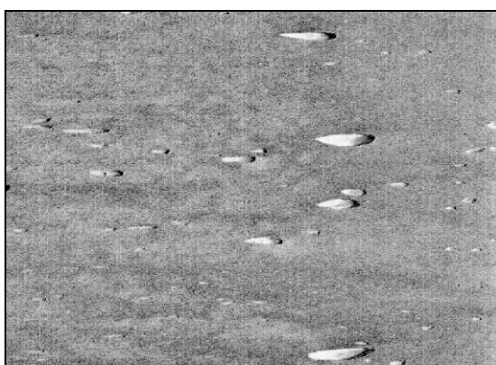
Figure 8a. Habitat type reef (1170). Sidescan picture showing scattered boulders on a flat, predominantly gravely seabed (reef type 3). The largest boulders in the picture raise 3-4 m above the seabed. Approximate dimension of the sections: Height 150 m and width 50m.
