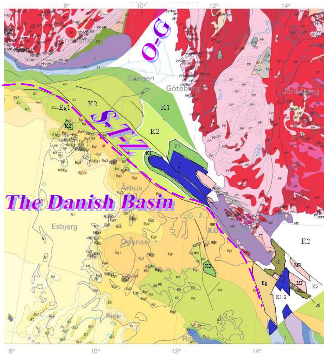
Figure 2. Pre-Quaternary map of Denmark. Red colours are Precambrian basement rocks at the margin of the Danish Basin. Blue colours are Jurassic and Triassic units, mainly occurring in fault blocks in the NW-SE striking Sorgenfrei-Tornquist Fault Zone (STZ). Green colours are Cretaceous chalk (K2), yellow-brown colour (EG1) is lower Tertiary limestone and marly clay. The light beige colour (N1) is Miocene sand deposits, which 15 million years ago formed a huge delta setting for the rivers draining the mainland of Europe out towards the North Sea. Between EG1 and N1, a number of clayey units appear mirroring the marine conditions under fluctuating water levels. O-G is the Oslo Graben, which is characterized by Permian volcanics. (Modified from Pedersen et al., 2002 and Pedersen, 2009).
