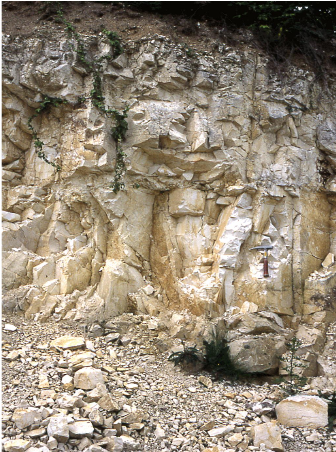
Figure 20. Danian limestone cut by horizontal and vertical fractures.
