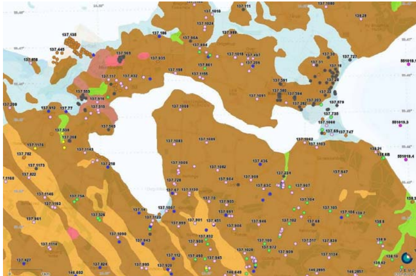
Figure 66. Map of the Quaternary surface deposits (From GEUS's Homepage. After Pedersen, 1989). Legend: Brown: Clayey till, red brown: Sandy till, red and orange: Melt-water sand and gravel, green: Holocene freshwater deposits, blue: Holocene marine deposits. Legend for boreholes: See fig. 67.
