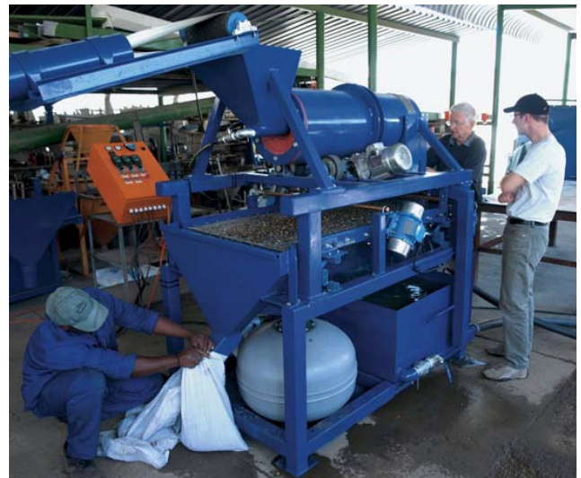
A test run with part of the modular plant: a high capacity, vibrating grease table, developed for Avannaa by Gondwanaland Diamonds, South Africa. Courtesy: Avannaa Resources.
